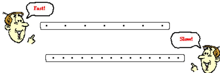
The analysis of a ticker tape diagram will also reveal if the object is moving with a constant velocity or accelerating. A changing distance between dots indicates a changing velocity and thus an acceleration. A constant distance between dots represents a constant velocity and therefore no acceleration. Ticker tapes for objects moving with a constant velocity and with an accelerated motion are shown below.
