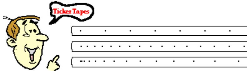
The distance between dots on a ticker tape represents the object's position change during that time interval. A large distance between dots indicates that the object was moving fast during that time interval. A small distance between dots means the object was moving slow during that time interval. Ticker tapes for a fast- and slow-moving object are depicted below.
